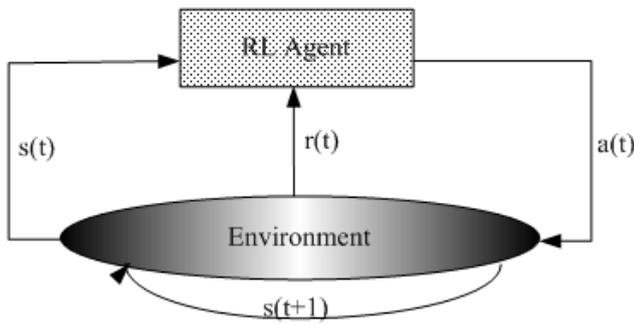
Fig. 2. Interaction illustration between an RL system and the environment
